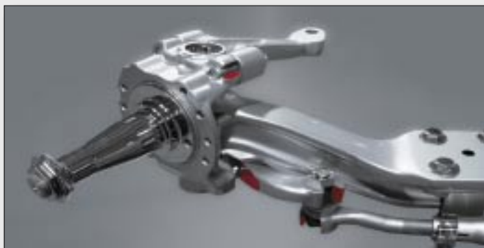
Steering and tie rod arms designed for maximum 55-degree wheel cut for added maneuverability.
